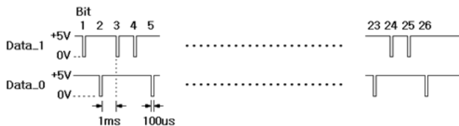
Figure: 26bit Wiegand Output Format
