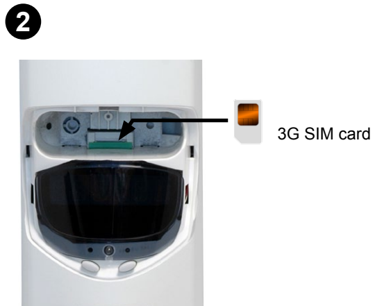
2 Insert the SIM card as shown. Push to lock. Push to eject.
