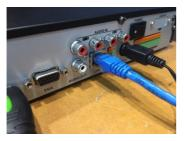
Attach the DVR to the network using the LAN port. The network should have a DHCP server (modem) to assign a network address to the DVR automatically.
